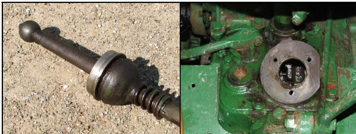
39-H Gear Shift Assembly (left) and Transmission Cover Port (right)
