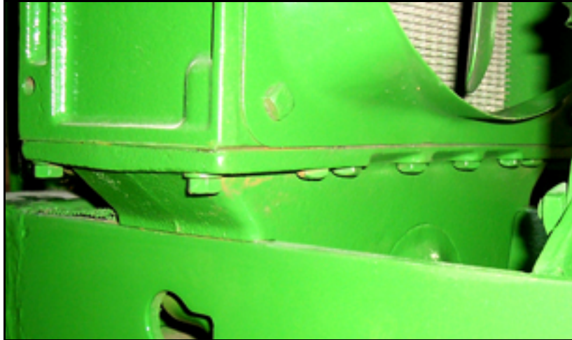
Fig 5. Bottom Rear-Side View – Note HCS at the Corner – Shown here w/lock washers
