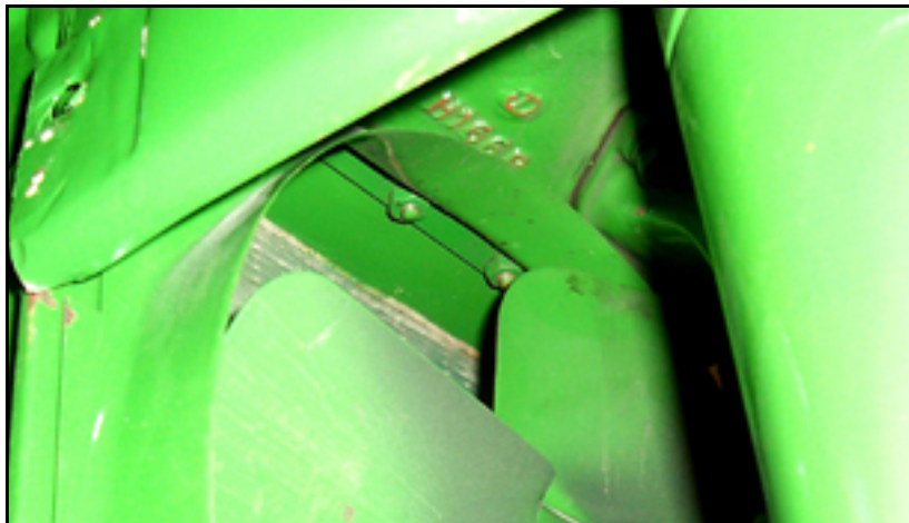
Fig 2. Top Rear View – Note Studs with Heavy Hex Nuts
