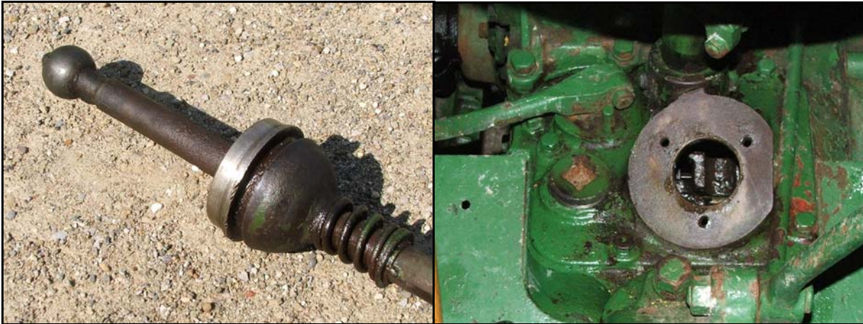
Figure 409 (D&E). 39-H Gear Shift Assembly (left), and Transmission Cover Port (right)
