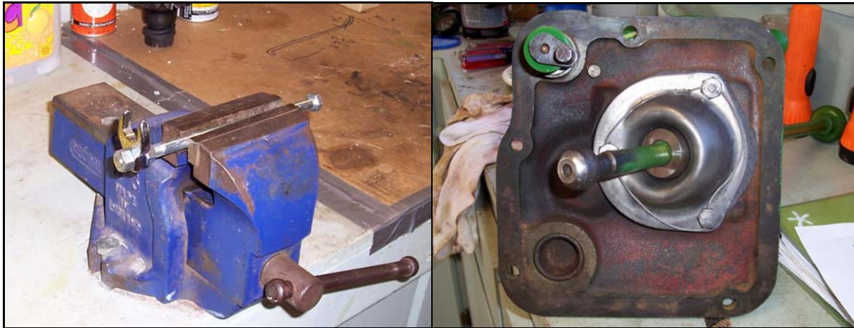
Figure 409 (A&B). Crowsfoot Wrench w/bolt, & Socket Safety-Wired in Place
