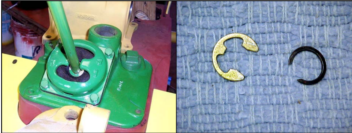
Figure 408 (A&B). External Clip EC-62 in Use, and Compared with B387R
