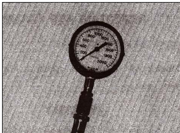
Fig 2-11 -- Gauge for Checking Pressure
