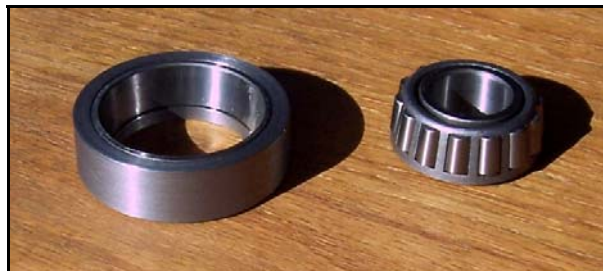
Photo of Tapered Roller Bearing – No Free/Floating Parts!
