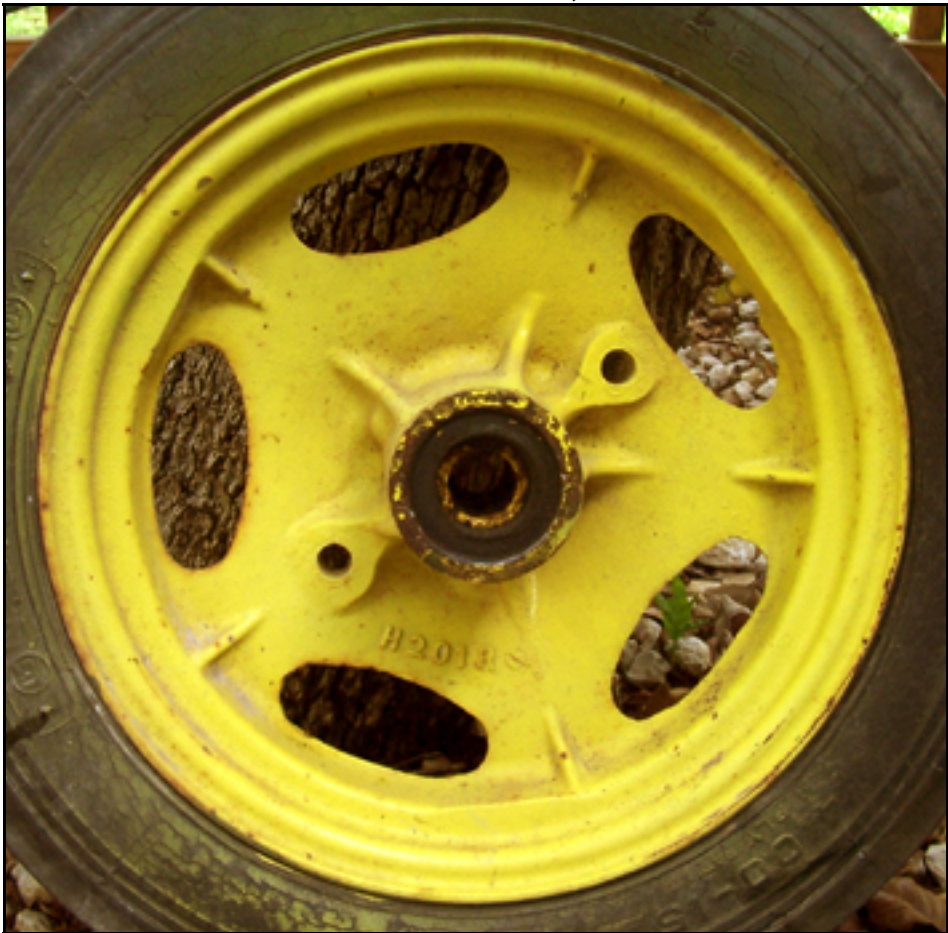
Earlier version cast (above) & later version of cast below (with ribs) - Inside View!
